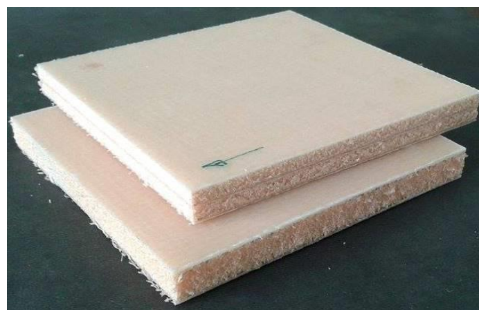
Figure 2. Prepared specimens of sandwich composites (a) with multi core (b) normal
